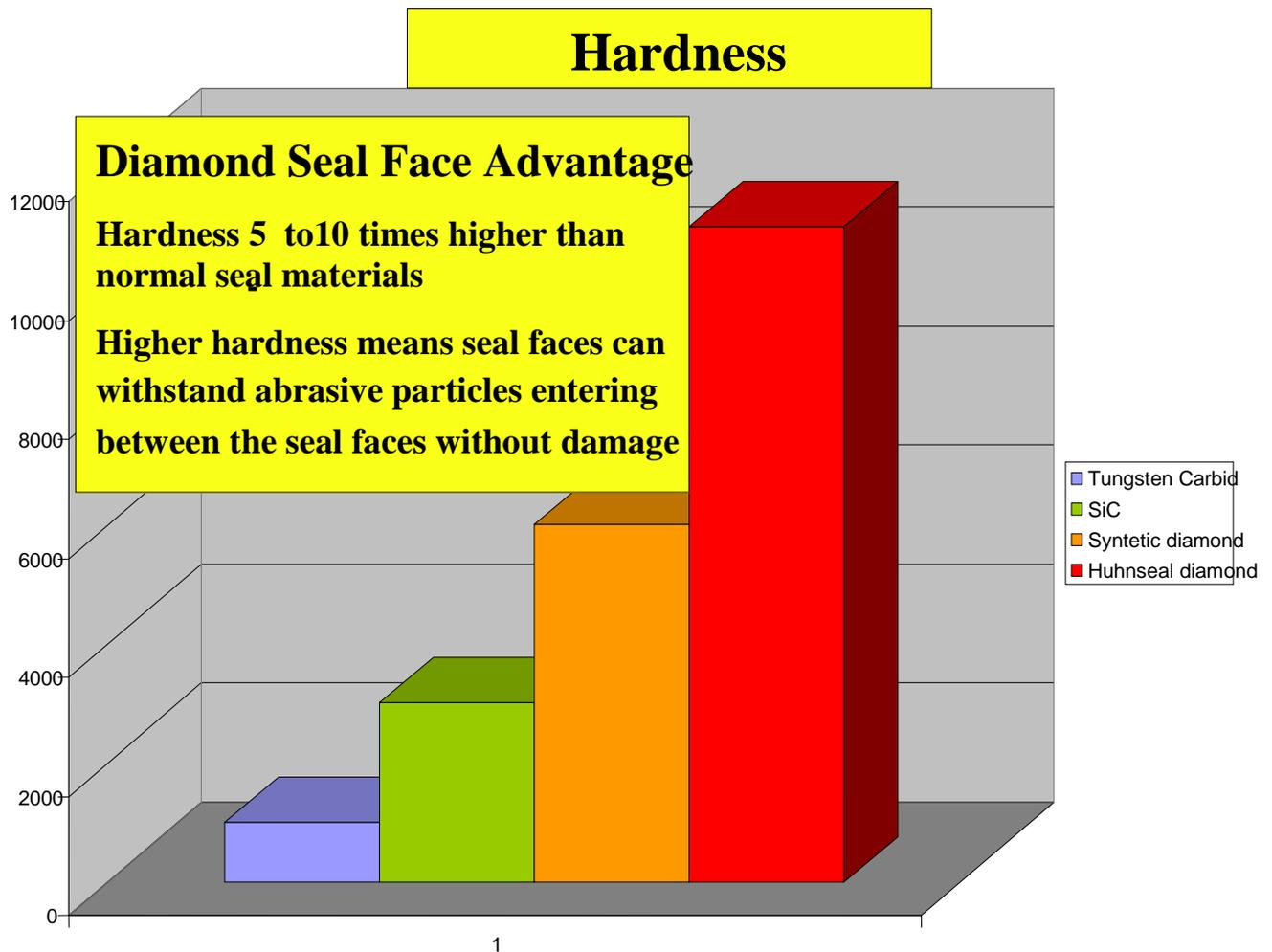
Diamond is the hardest substance known to mankind. With this kind of hardness, the seal faces simply pulverize any solid material that enters the seal faces. This allows pumping of clay or metal slurries without the need for expensive double seal systems and their resulting operation difficulties. In many cases, the need for water requirements to make the seals last in service is no longer required.
