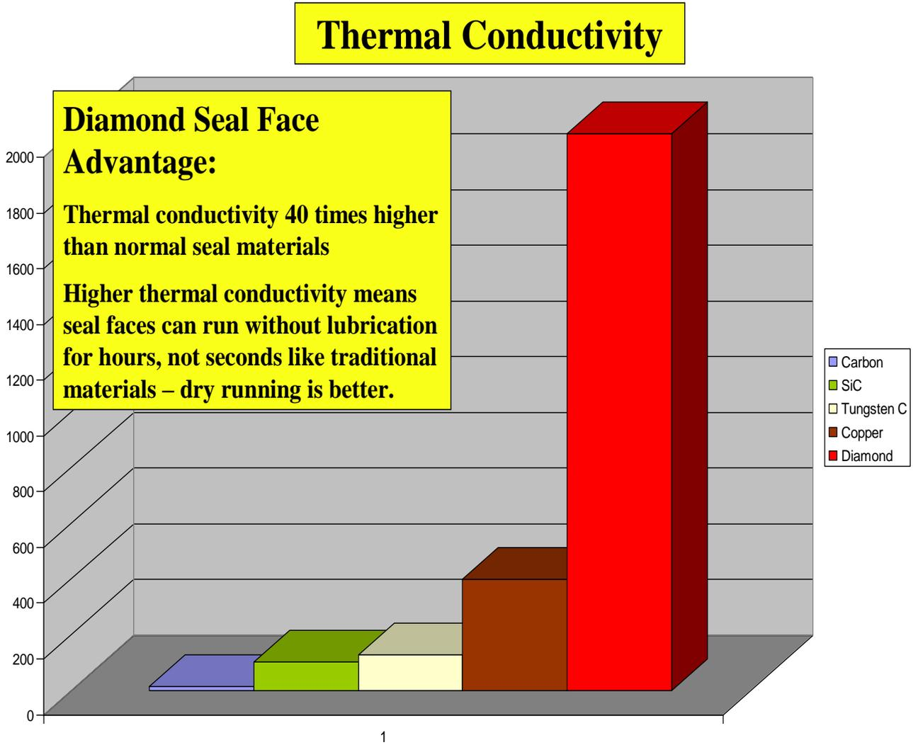
The low coefficient of friction along with the extremely high thermal conductivity of the diamond means that the little heat generated at the seal faces is quickly dissipated away from the seal faces.
