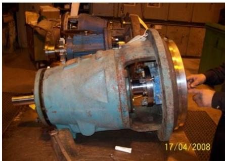
Huhnseal Diamond Seal being Installed on a Goulds 3175 Pump
