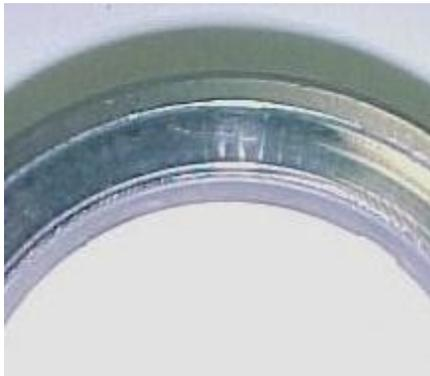
Dry running causes thermal cracking of seal faces and burning of the elastomers.
